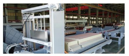
This device is installed in the upper part of filter press. It's made up of washing rail, washing frame, washing frame driving travel device, inlet pipe, towing chain, washing pipe, nozzles, washing pipe lifting device, reducing motors etc. It can finish cloth washing in co-operation with plate shifting device under the control of PLC. This system makes it possible to wash the cake residues off the cloth using water under pressure. Washing is performed simultaneously on both sides of the plate.
